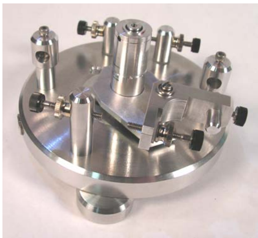
This is the bell-crank mechanism mounted on its carrier, which then mounts to the central pillar, as shown below.
