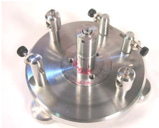
The magnet holders, contacts, and the rotor rest stop are mounted on the base.
