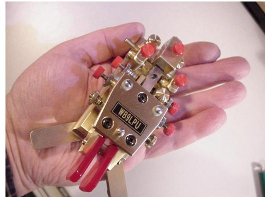
While it is tiny, this bug (which also can function as an iambic paddle) is very stable and works like its larger cousins. Because of the need for stability, only brass will be used in its construction - a wooden base might not be steady enough.
