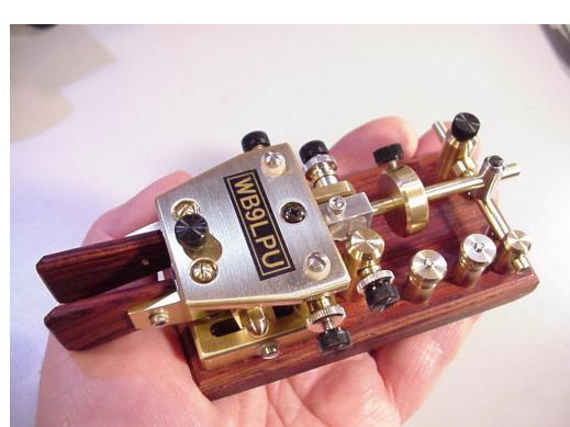
This can also be built from the same variety of materials as used before. Because of the different magnet system, the paddle-arm springs must be magnetic.
