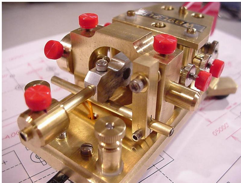
The switch cylinder is mounted to the fixed magnet holder through a vertical bar with a rod-clamp arrangement at the bottom. While this approach allows a full range of adjustment in two planes, it is rather easily disturbed because the lock mechanism is too far away from the tip of the tube.
