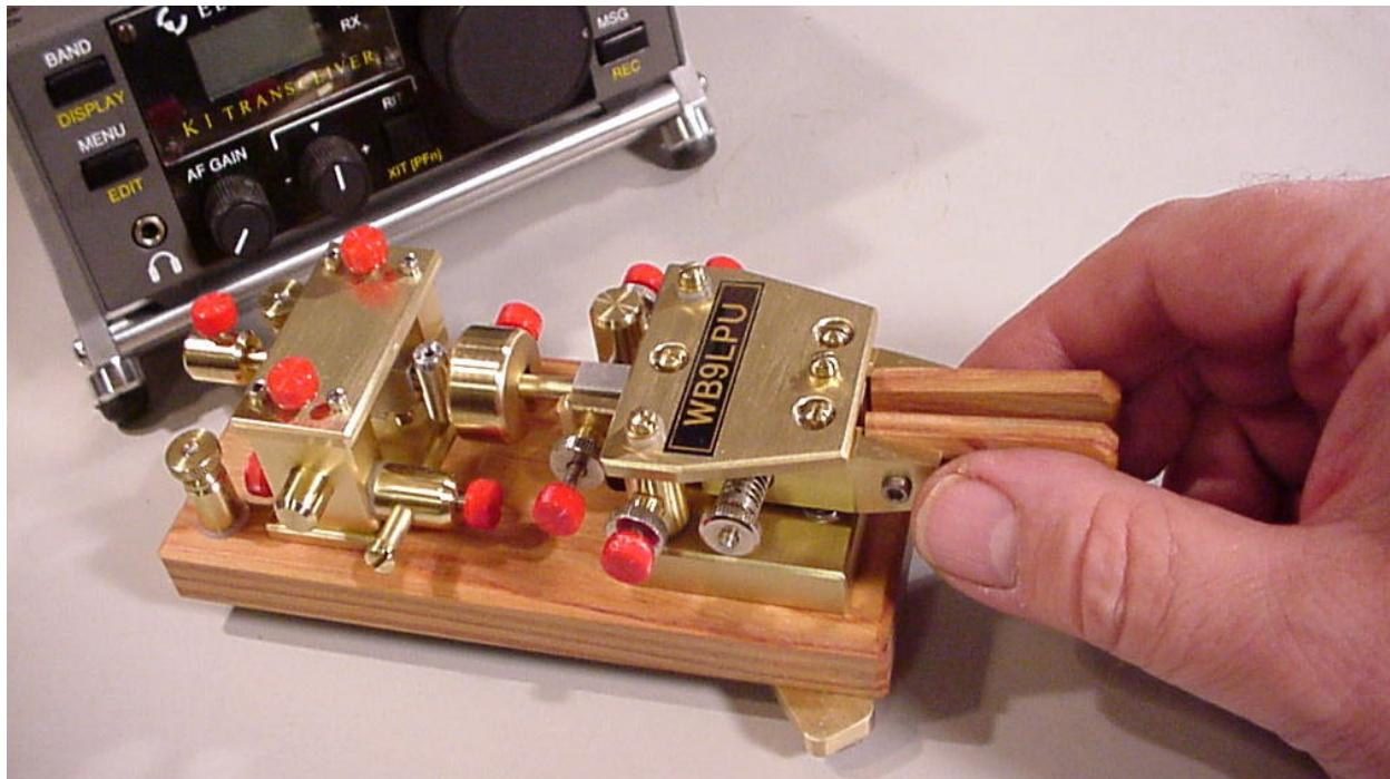
The Parkwood PaddleBug, shown here as prototype #1, is part of the ongoing design of keys, paddles, and bugs at WB9LPU. This device is another step in the investigation into the design and construction of magnetically-controlled bugs and it uses an approach not found in its predecessors.
