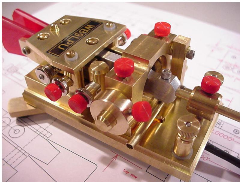
The circular object in the foreground is a "place-keeper" for the right magnet. Withdrawing this magnet causes a constant deflection of the pendulum to its rest position, and the unit then functions as a conventional paddle. The placekeeper allows the unit to be returned to its "bug" function without loss of its adjustments.
