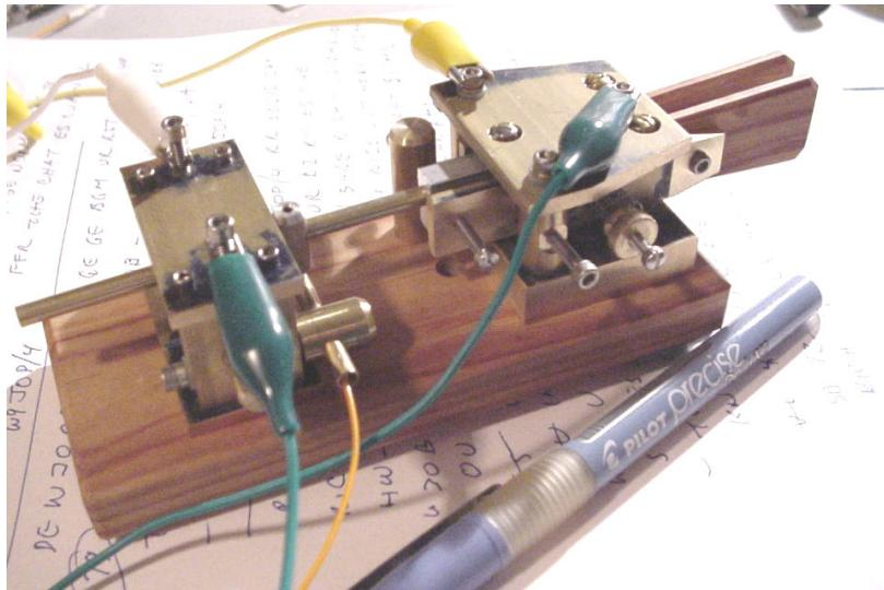
At an early stage of testing, the unit is connected up with alligator clip leads. Even at this early stage, it gave a good account of it on the air (thanks to the patience of the ham on the other end of my "new-bug fist.")
