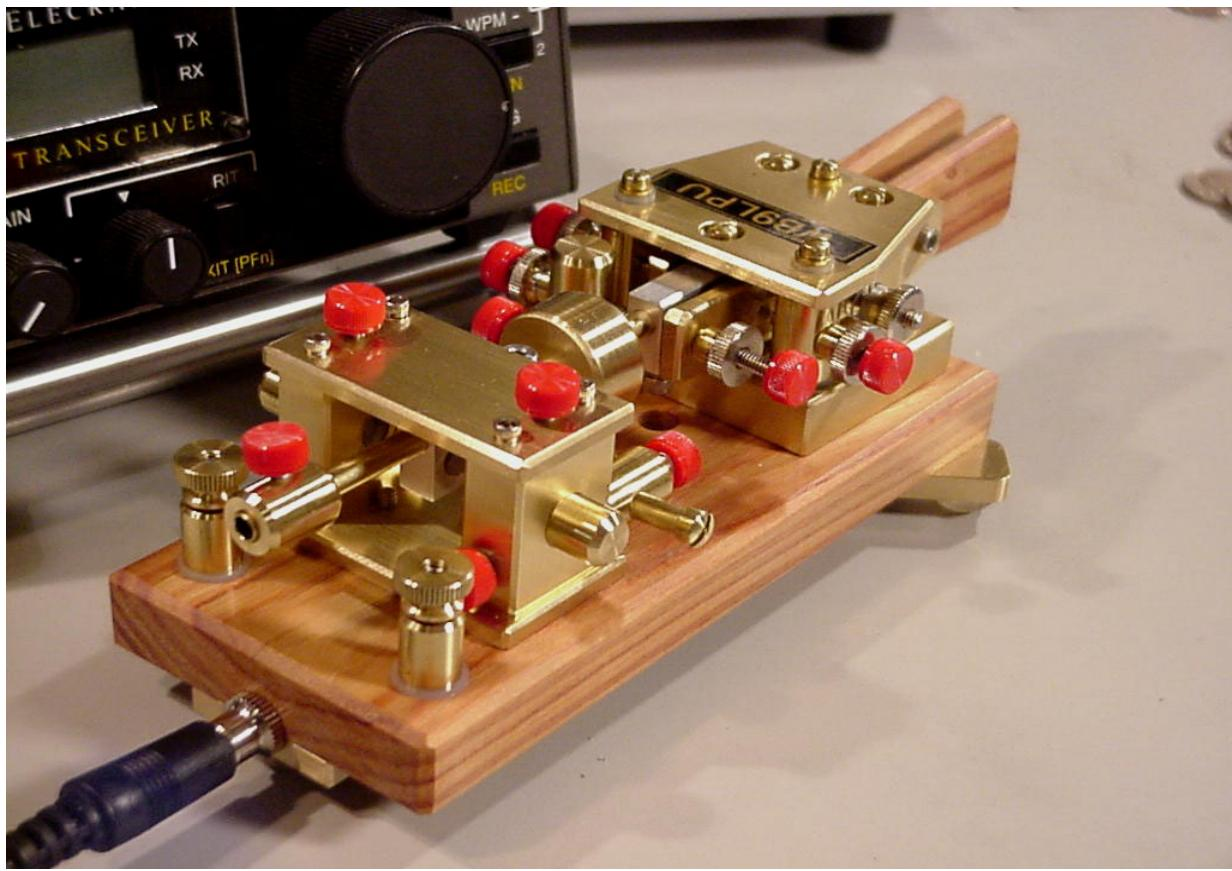
The PaddleBug is a nice size for a small operating position (read “cluttered desktop” in my case). In this view, the two magnets that make the pendulum oscillate are seen protruding from the assembly with the two locking screws on top. The smaller pendulum weight extends between the binding posts.
