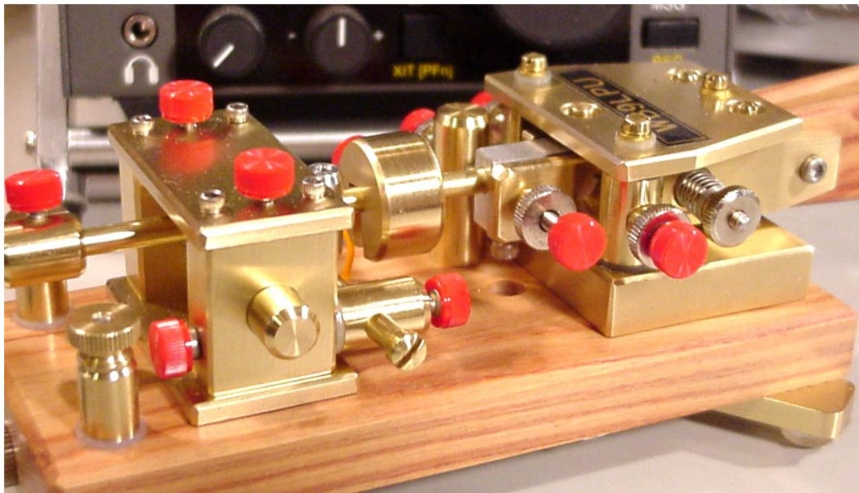
In this side view, the reed switch holder is at the lower center. The switch position can be changed to compensate for changes in the position of the pendulum, or to change the "weight" of the "dit" stream.
