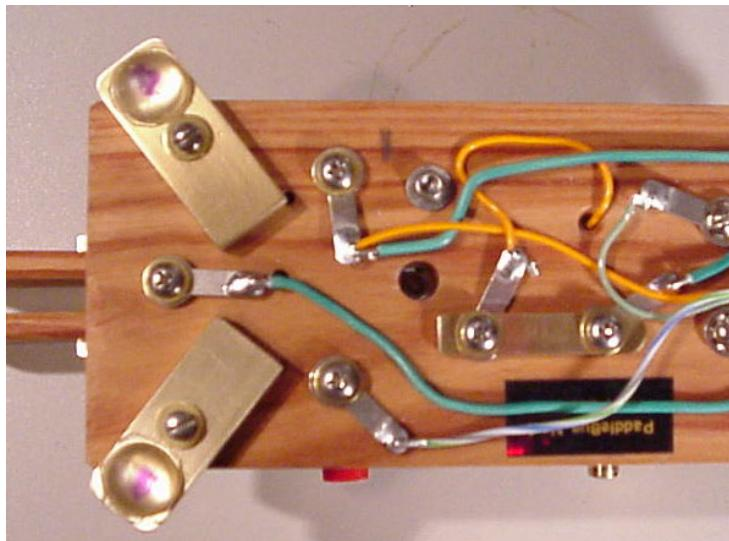
The brass link seen near the middle of the bottom removes the reed switch from the circuit to disable the bug function and leave the paddle operation intact. The same result can be obtained by restraining the movement of the pendulum. In future versions there will be a mechanical stop for this function.
