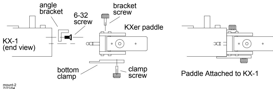
This drawing shows on method of mounting the paddle. The angle bracket is first mounted to the KX-1, then the paddle is plugged in and the bracket is secured to the paddle with the bracket screw. The bottom clamp holds the paddle securely and eliminates any movement while the paddle is in use.
