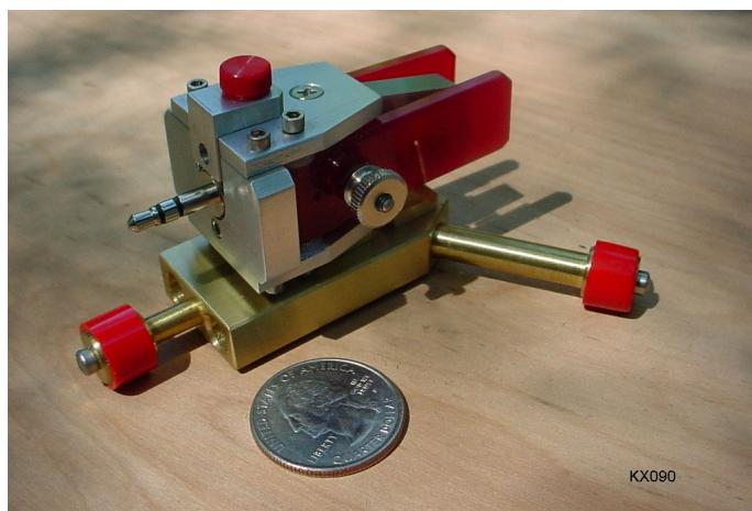
In its stand-alone mode, the tripod legs provide stability, and the brass base provides just enough weight so that the paddle doesn't move (with a moderately light touch). The paddle is raised slightly above the base by using the bottom clamp as a spacer.
