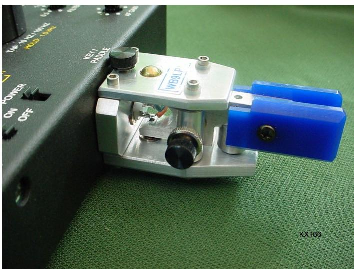
The single paddle prototype mounted to the KX-1. This version uses a ball-bearing below the paddle arm and a single brass ball above the arm. The "wobble-toggle" spring assembly is just below the front of the fingerpieces. Contact spacing is set by the black knobs, which can be locked. The paddle mounting uses a variation of the bracket method, substituting a 6-32 stud for the bracket and holding it with the upper
