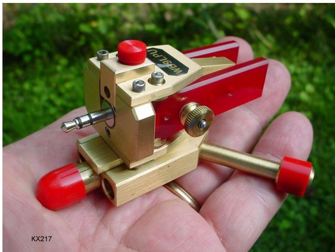
This is an all-brass version, mounted on its base. It uses 3/16" brass balls for bearings and is very smooth in action. The brass construction makes it a bit heavier than the aluminum model, which provides a little more stability when it is standing alone. Here the bottom clamp is used as a spacer.
