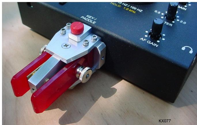
Here is the paddle mounted to the KX-1. The brass contact strip may be seen on the inside of the dot-paddle.
