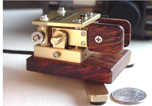
A brass paddle with short fingerpieces, mounted on cocobolo wood
