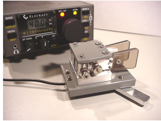
This aluminum and steel paddle, with spring tension, is styled to match a popular transceiver.
