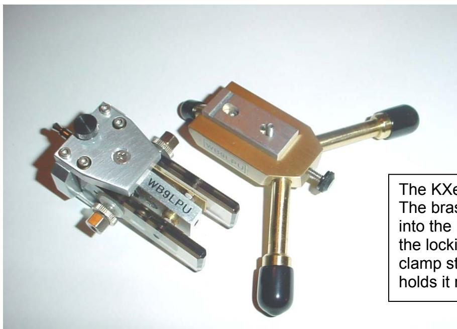
The KXer and its mounting parts. The brass screw has been threaded into the KX-1 and will be gripped by the locking screw. The rectangular clamp stabilizes the paddle and holds it rigidly in place.
