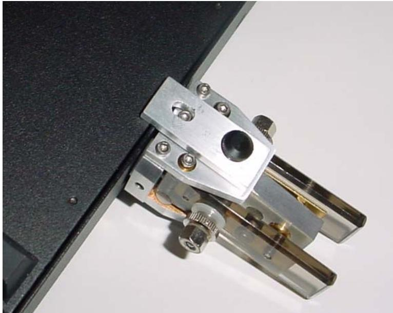
This view shows the under side of the paddle with the bottom clamp in place. Its groove should be engaged with the front of the KX-1 housing.
