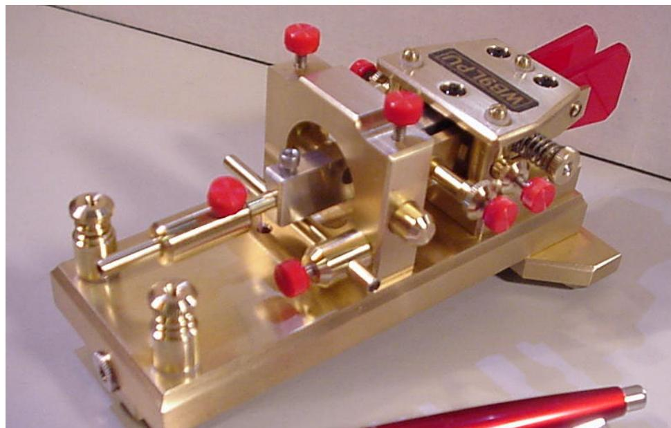
The PaddleBug is a nice size for a small operating position (read "cluttered desktop" in my case). In this view, the two magnets that make the pendulum oscillate are seen protruding from the upright assembly with the two locking screws on top. The brass tube containing the reed switch runs below the pendulum, and moving it back and forth allows setting of the duty cycle (dot-to-space ratio) of the "dit" stream.
