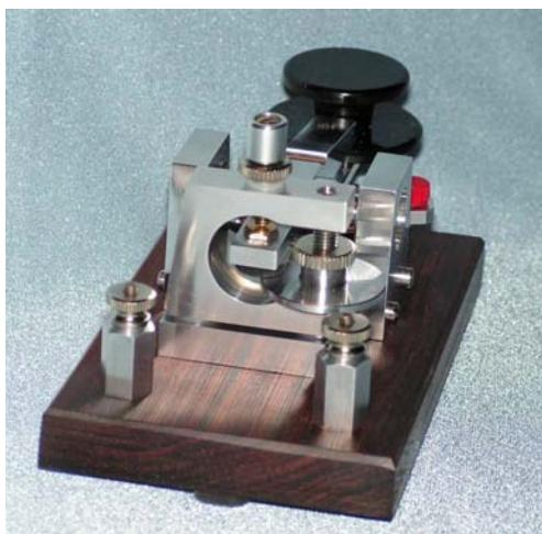
This is a close-up of the spacing adjustment mechanism. One side of the trapezoid is cut away to allow a 10-32 threaded rod to carry the rest stop.
