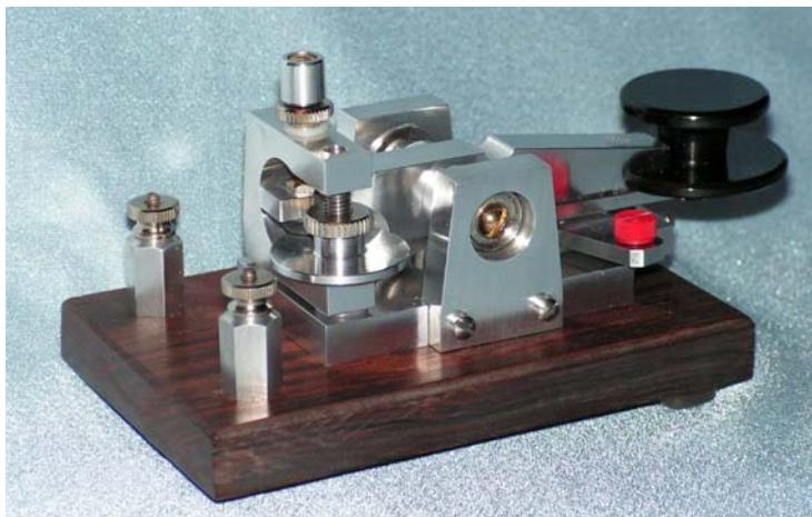
This key is significantly shorter (some might call it "dumpy"), but it has a nice feel and is very quick and solid in its action. The red knob moves the magnet slide, and the lock is on the other side of the small adjustment lever.
