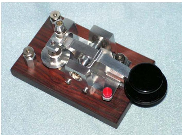
This top view shows the bearing assembly and all of the adjustment mechanisms. All of the parts of the key are mounted on an aluminum frame which is in turn mounted on the wooden base.
