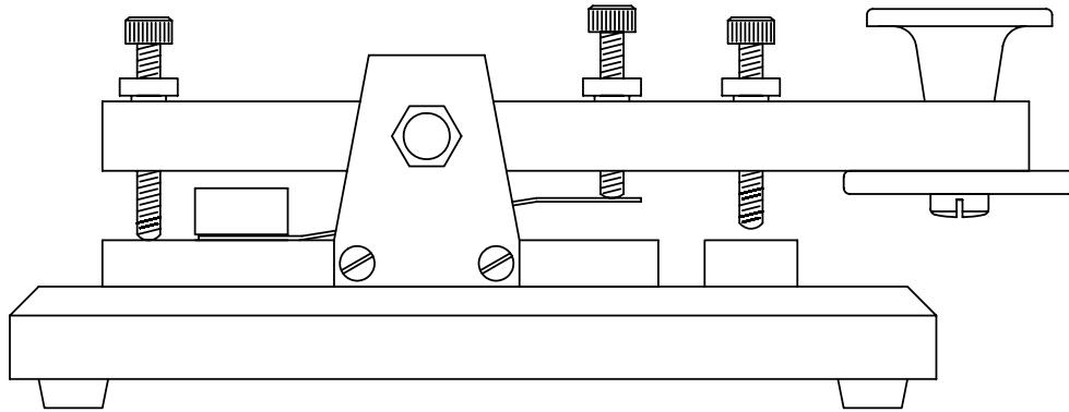
This project was designed to illustrate the kind of results that you can obtain by combining careful work with simple tools. While most home hobbyists (of the ham radio variety) do not have a milling machine or lathe, many typical home workshops contain all of the tools necessary to produce very good work. The key described here was made using a drill press, a belt sander (optional), and various common hand tools.
