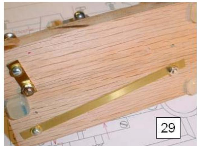
screw hole to locate the lower contact pad shown just to the rear of the main baseplate. Drill the holes as before; one mounting screw must be long enough to pass through the wooden base to make the electrical connection.
