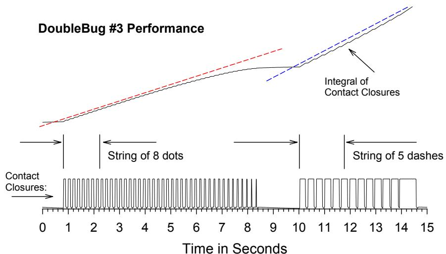
Shown below is an off-the-air recording of the waveform of a CW message. The errors in timing are primarily those of the operator, not the instrument.
