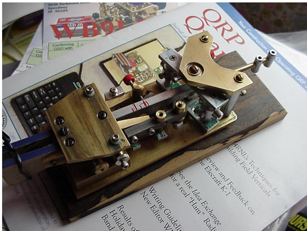
So the next design retained the one-side single- pendulum idea, but rotated the magnetic field to weaken it and produce dashes. This solved the paddle-force problem, but not the momentum problem. It also used a very complex set of linkages that was tricky to adjust and noisy in operation. This
