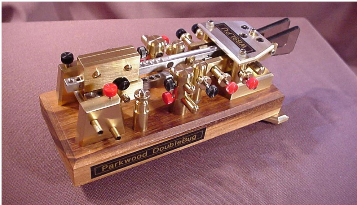
The next attempt used over-and-under pendulums with side-by-side bearings. The magnet holders were redesigned to make adjustments more accessible, and more room was allowed for the sliding weights. This produced a key that was easy to adjust and use - it feels like a conventional paddle with a fairly large travel of the dot and dash levers. The elements (dots and dashes) are not self-completing, so a little care must be taken.
